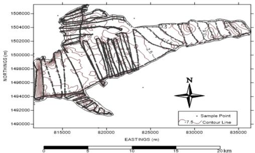
**Figure 3:** Current Bathymetric Map of Goronyo Reservoir Generated by Surfer 11 **Source:** (Authors, Field Work, 2013)
